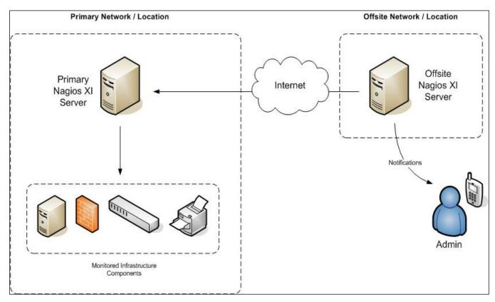
With this type of monitoring architecture, a second Nagios XI instance is installed at an off-site location or separate network. This off-site location can be a home office or a data center in a separate geographic location.
