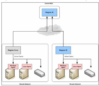
Nagios administrators that have large remote networks, or that require complex or in-depth monitoring of remote network elements may choose to deploy a federated monitoring architecture.
