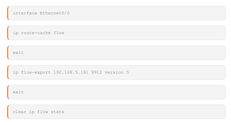
Now all traffic flowing through interface Ethernet0/0 will be analyzed by the Cisco device and will be sent to the Nagios Network Analyzer for further processing. Be sure to save the configuration once you've determined proper functionality of exporting the Netflow data.
