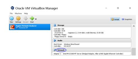
You need to select what network the network adapter is connected to.
