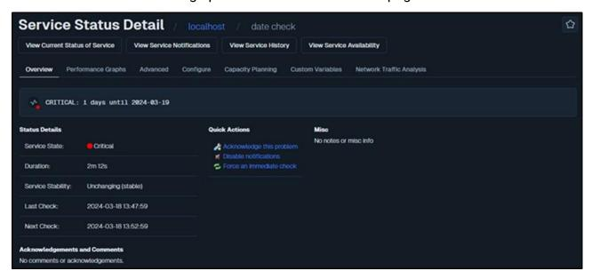
In this screenshot, you can see that the service has the same output that the test in a terminal session produced, so we know the service is correctly working. This means that the new plugin that was added to Nagios XI is working as expected.
