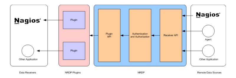
NRDP has the capability of allowing remote agents, applications, and Nagios instances to submit commands and host and service check results to a Nagios server. This allows Nagios administrators to use NRDP to configure distributed monitoring, passive checks, and remote control of their Nagios instance in a quick and efficient manner.
