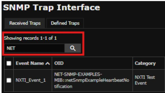
The screenshot shows the 'SNMP Trap Interface' with tabs for 'Received Traps' and 'Defined Traps'. A search bar contains the text 'NET'. Below the search bar is a table with the following data:
