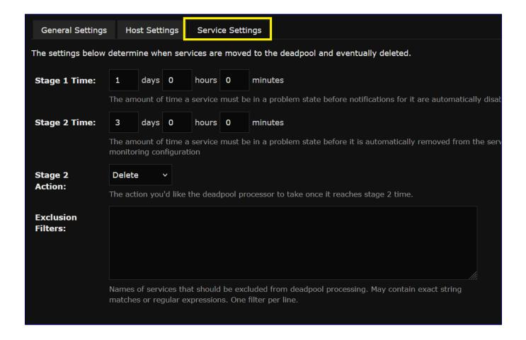
**Stage 1** determines how long an object must be in a problem state before notifications are disabled, and the object is added to the deadpool.
