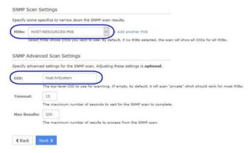
The **MIBs** list allows you to limit the results of your scan to one or more MIB files. In this example I have chosen the HOST-RESOURCES-MIB file.
