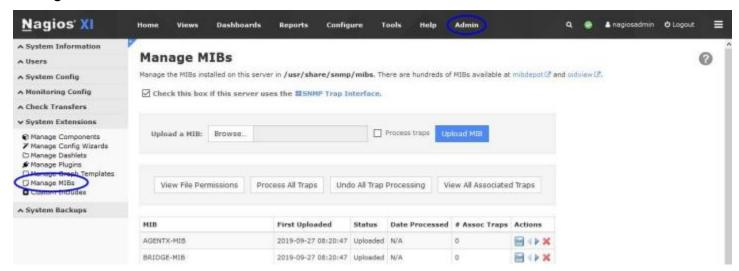
You can use the **Browse and Upload MIB** buttons to upload your own MIBs. Understanding how to read a MIB file can help you get the most out of the SNMP Walk wizard, however it's not required knowledge at this point. The **Understanding MIB Files And Objects** section in this documentation does explain how to read a MIB file which may be of some help.
