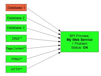
For this particular business process, a redundant database solution is being used for a web service. If one of the 3 database servers goes down, there are two more servers in place to act as fail-over solutions. Even though the first server is in a critical state, the actual business process of the web service is still in an OK state because all services required for it to run correctly are still in place.
