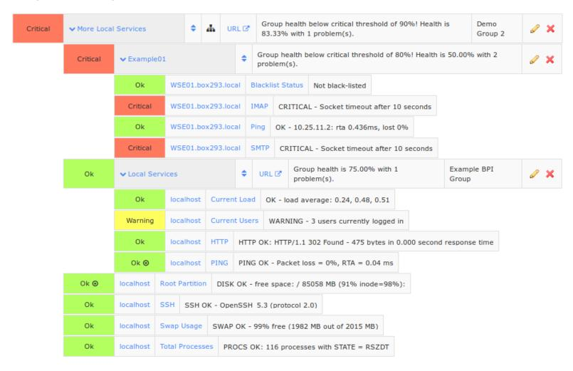
The BPI groups determine state by looking down only one level. The BPI group will essentially look for the worst state trigger in the group, so if the warning threshold is exceeded for a group, but an essential member is "critical", the group will still be "critical".
