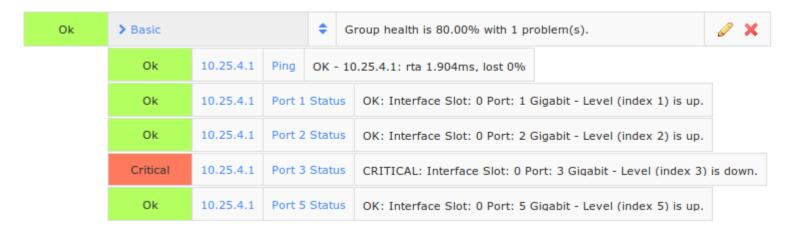
This is a basic group with 5 members. The group has a *warning threshold* of 70%, and a *critical threshold* of 60%. Even though the group has one member in a Warning state, the group state is still 'OK' because the health percentage is at 80%.
